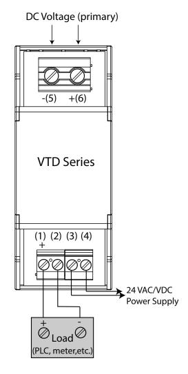
Note: No isolation between power supply and output signal connections.
