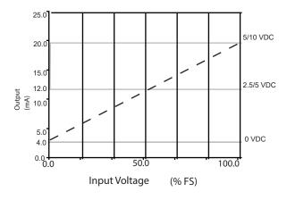
Note: Voltage output will be linear in the same manner, with zero at zero primary voltage and 5 or 10 VDC at the full range measured voltage.
